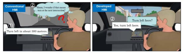
Comparison of conventional navigation system and newly developed HMI's "natural navigation"
