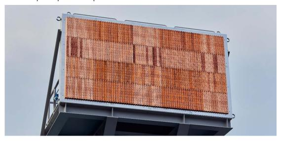
Prototype of resin-injection-molded waveguide array antenna
