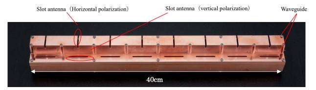
Close-up of slotted waveguide array antenna
