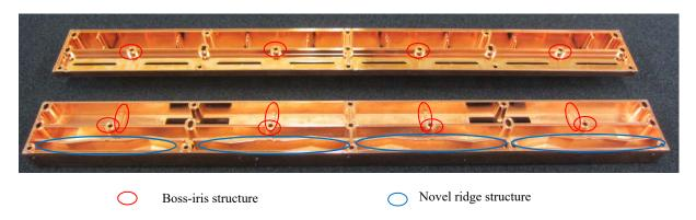
Inside of Close-up of slotted waveguide array antenna
