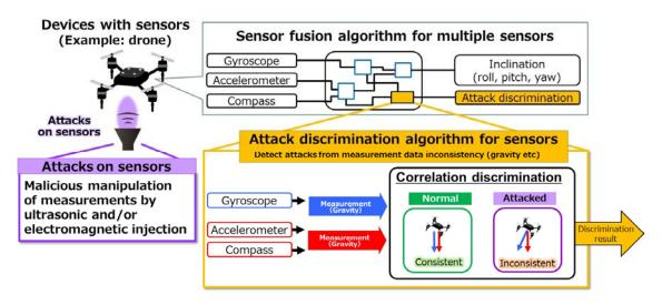
Application example using a drone
