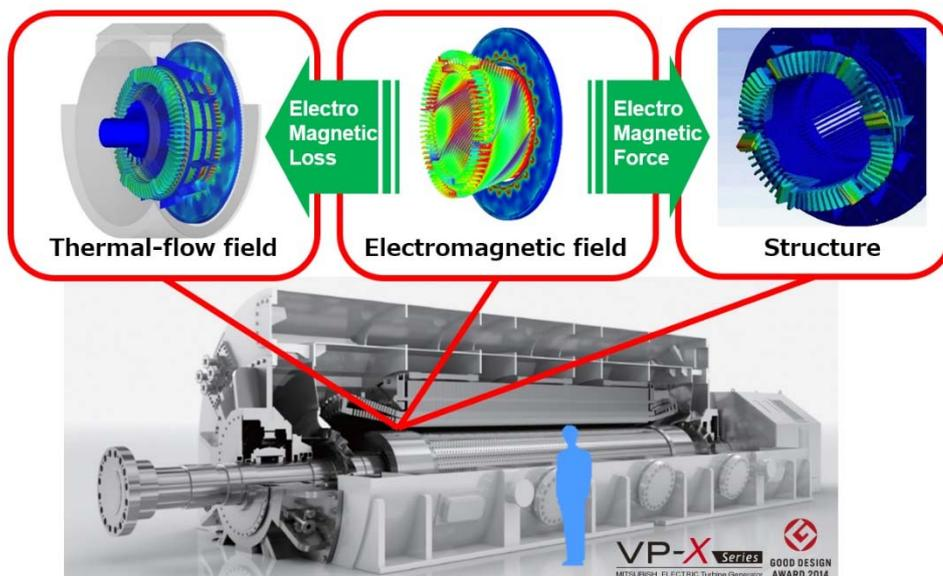
The technology analyzes the interaction between electromagnetic-field and thermal-fluid-flow-field, as well as the structural configurations of power generators, enabling the detailed distribution of temperature and vibration to be calculated based on detailed loss distribution and electromagnetic force.
